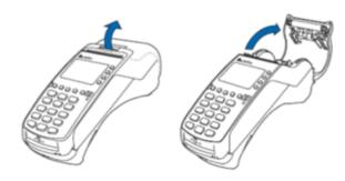
» Place paper roll into the well, with paper coming up from the underneath of the roll, leaving at least one ("1") inch outside of the well
